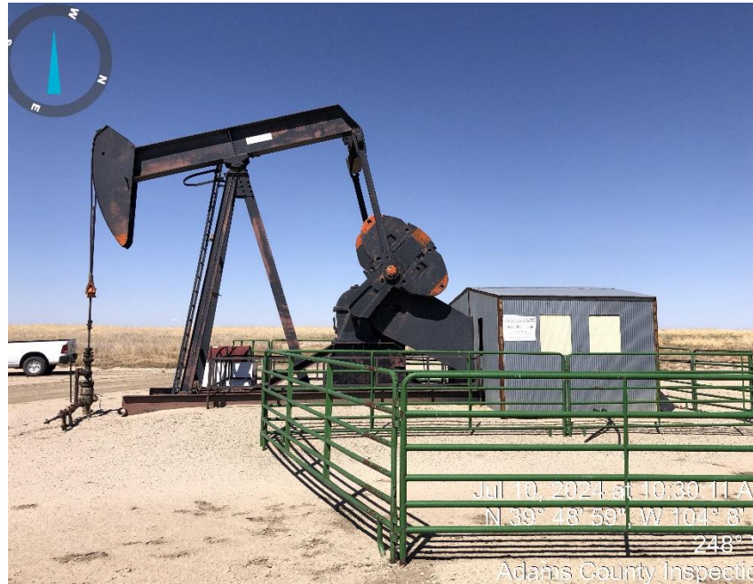
Photo #1 Pump jack.
