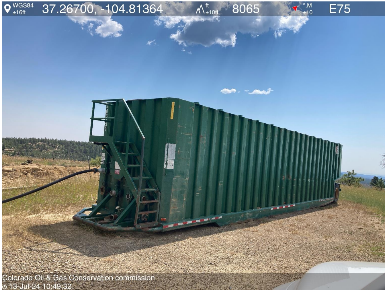
PHOTO 4: UNUSED EQUIPMENT LEFT ON LOCATION (FRAC TANK). REMOVE UNUSED EQUIPMENT PER RULE 606. CA DATE 8-13-2024.
