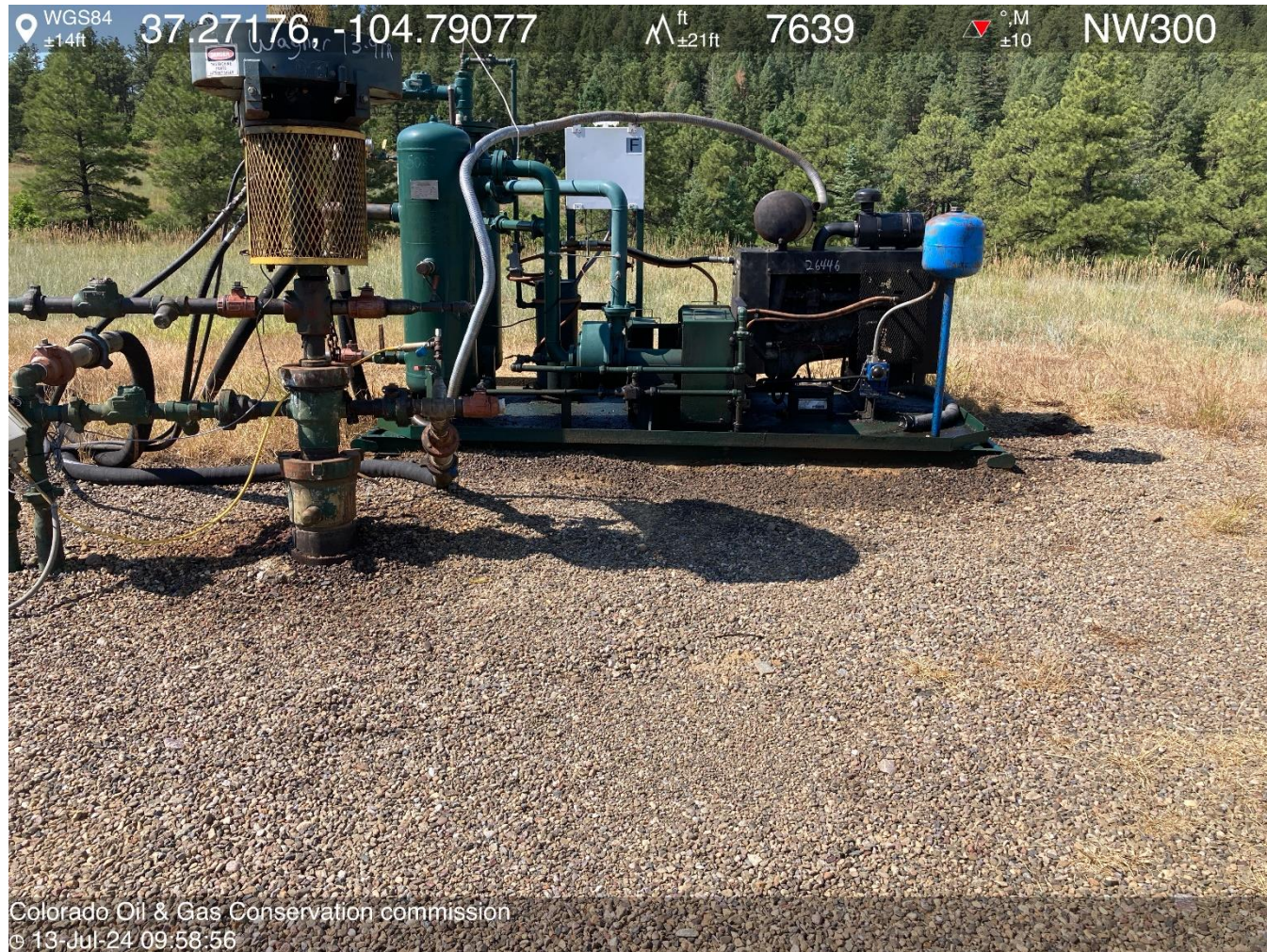
PHOTO 4: AREA OF IMPACTED SOIL AROUND COMPRESSOR SKID, COMPRESSOR IS COVERED WITH A FILM OF OIL ALL OVER THE EQUIPMENT INDICATING SEVERAL LEAKS. REPAIR OR REPLACE LEAKING EQUIPMENT, REMOVE OR TREAT IMPACTED SOILS, Self-inspection, maintenance, and good housekeeping procedures and schedules PER RULE 1002..(2).D. CA DATE 8-13-2024.
