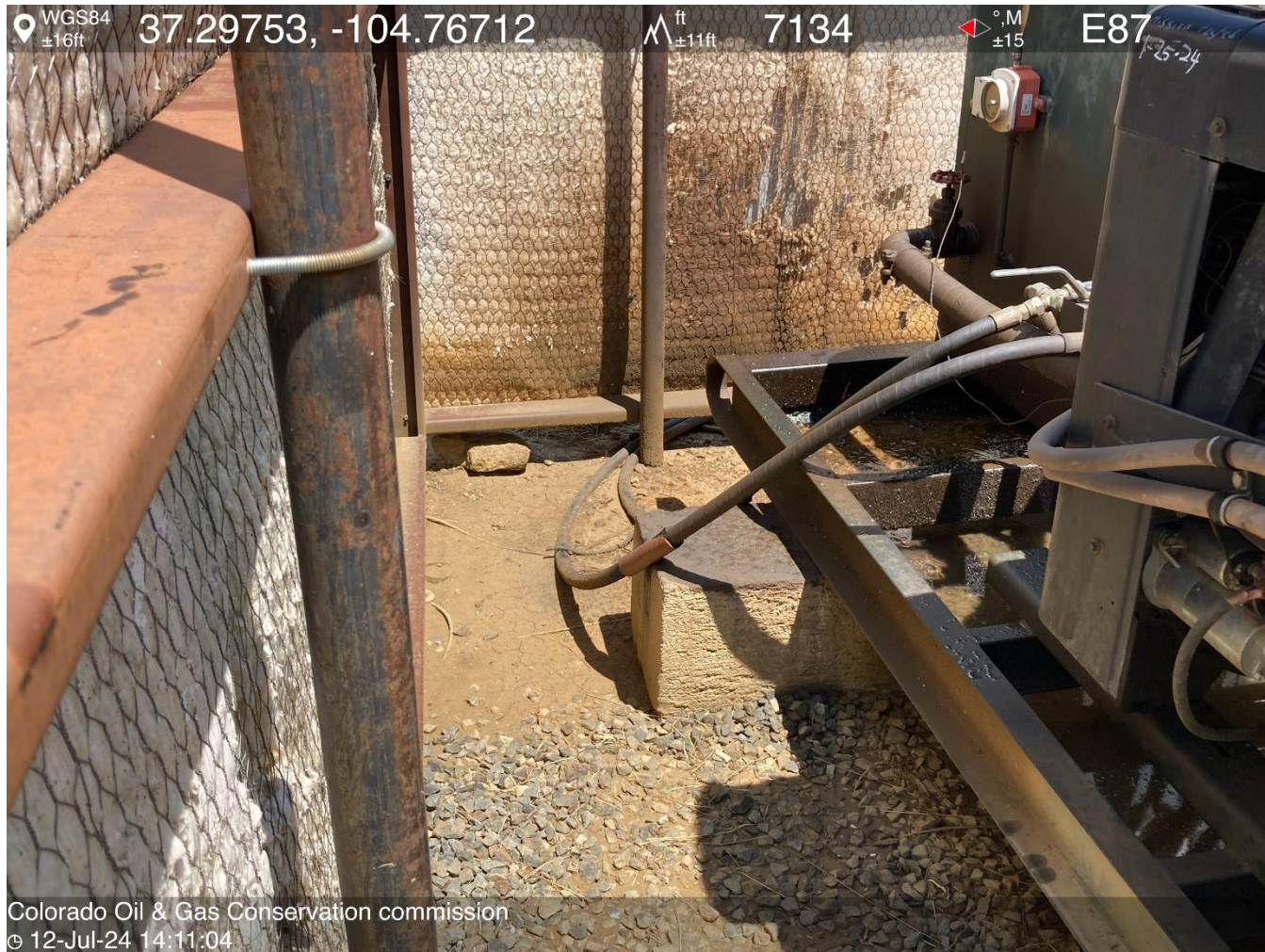
PHOTO 5: OILY WASTE IN PRIME MOVE SKID HAS SPILLED OVER CAUSING IMPACT SOIL SURROUNDING SKID. REPAIR ALL LEAKS AND REMOVE OR TREAT IMPACTED SOIL PER RULES 1002..(2).D. CA DATE 8-13-2024.
