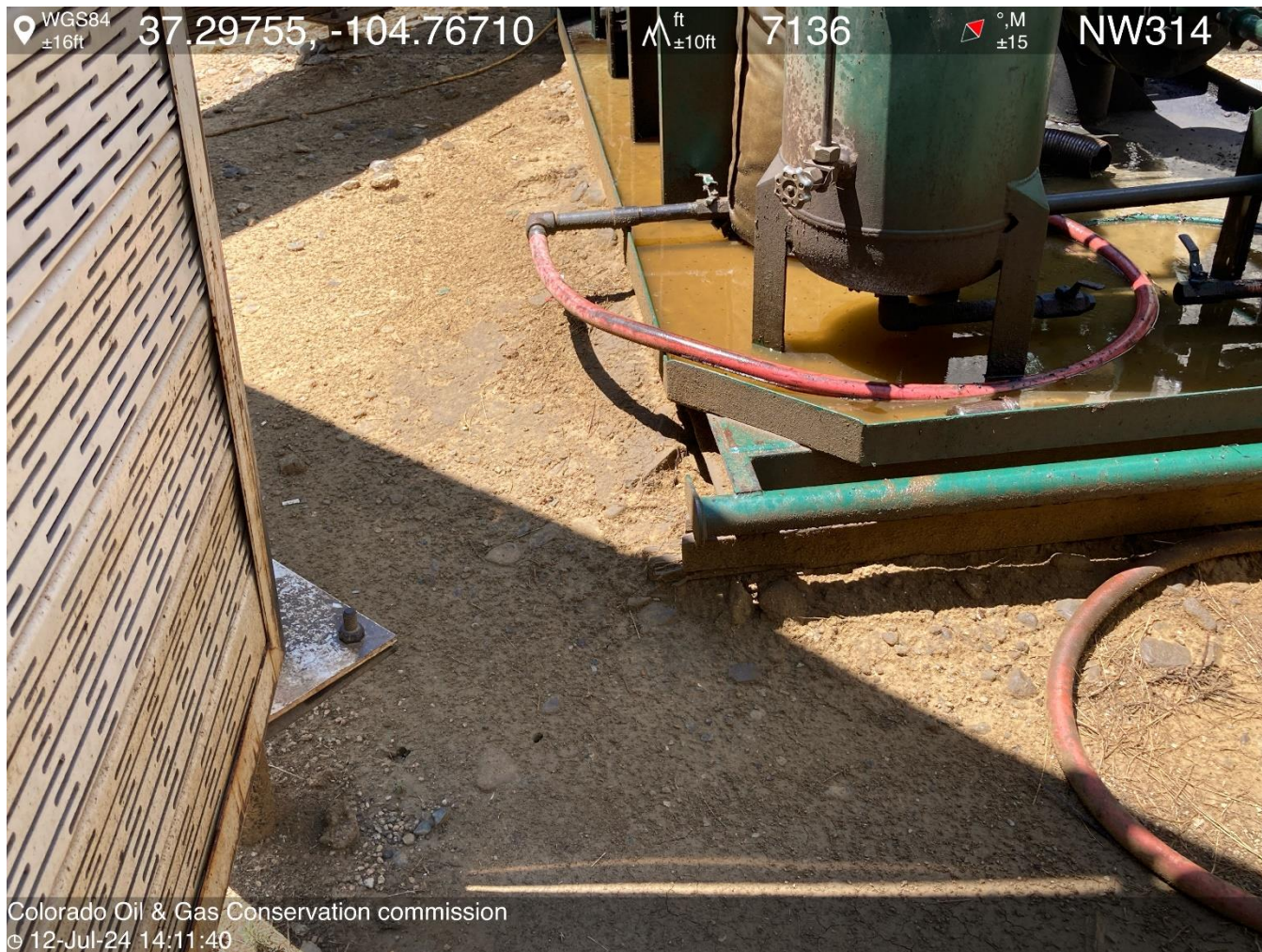
PHOTO 6: OILY WASTE IN COMPRESSOR SKID HAS SPILLED OVER CAUSING IMPACT SOIL SURROUNDING SKID. REPAIR ALL LEAKS AND REMOVE OR TREAT IMPACTED SOIL PER RULES 1002..(2).D. CA DATE 8-13-2024.
