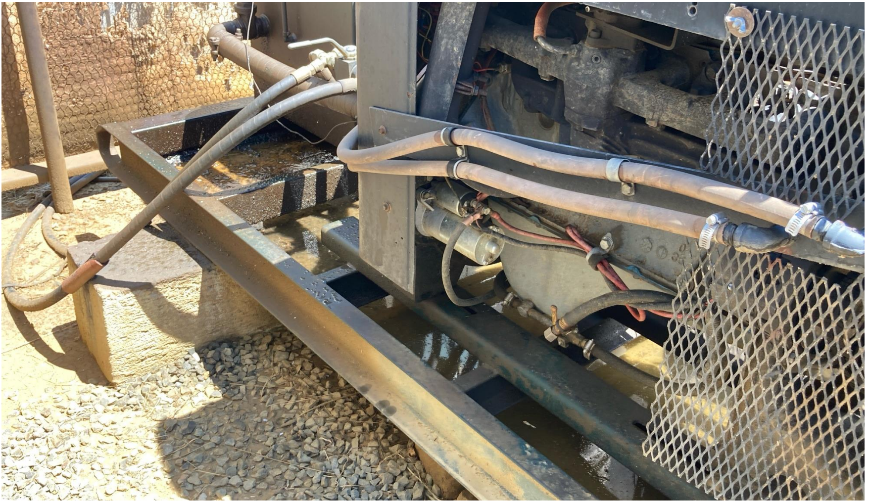
PHOTO 4: OILY WASTE IN PRIME MOVE SKID HAS SPILLED OVER CAUSING IMPACT SOIL SURROUNDING SKID. DRAIN OILY WASTE REPAIR ALL LEAKS AND REMOVE OR TREAT IMPACTED SOIL PER RULES 1002..(2).D & 1002.f.(2)B, Comply with general provisions of the oil and gas act for wildlife protection AND SB-181. CA DATE 7-13-2024.
