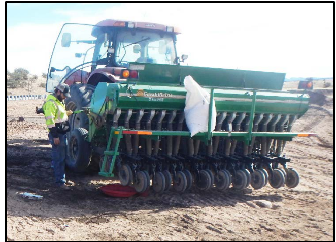
Drill Seeder Calibration
