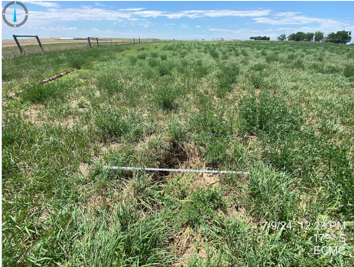
Photo 9. Subsidence observed at one of the flowline potholes.
