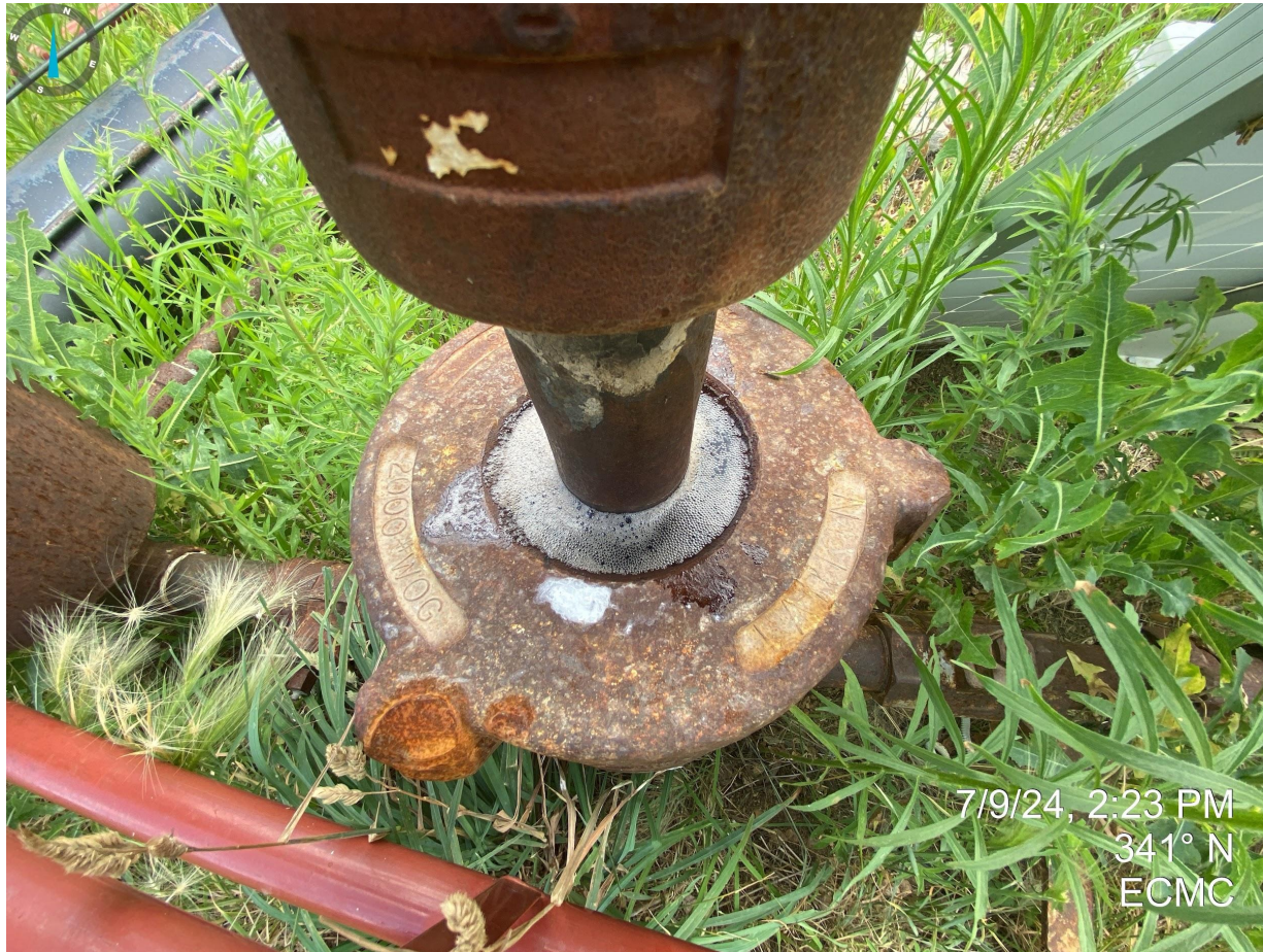
Photo 1. Venting observed as bubbles in standing fluid at casing assembly.
