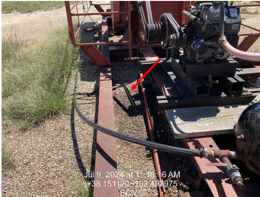
Photo 3 – Oil Stains in pumping unit frame
