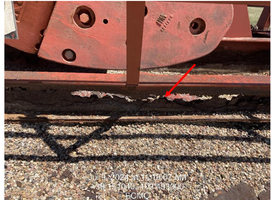
Photo 4 – Pumping Unit base is corroded.
