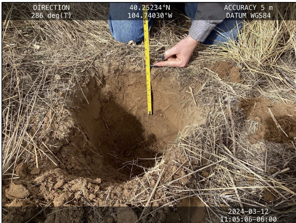
Photograph 6. Topsoil depth pit (CS06) – showing a change in color and hardness at 7 inches .
