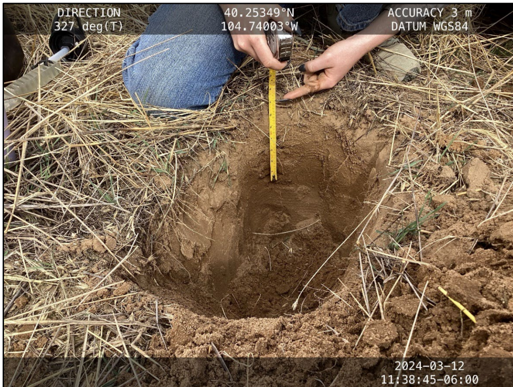
Photograph 1. Topsoil depth pit (CS01) – showing a change in texture and hardness at 7 inches .
