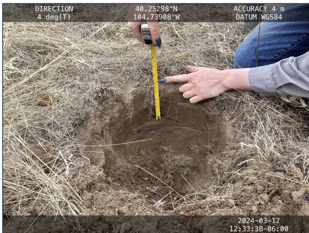
Photograph 3. Topsoil depth pit (CS03) – showing a change in color and lack of roots at 5 inches .
