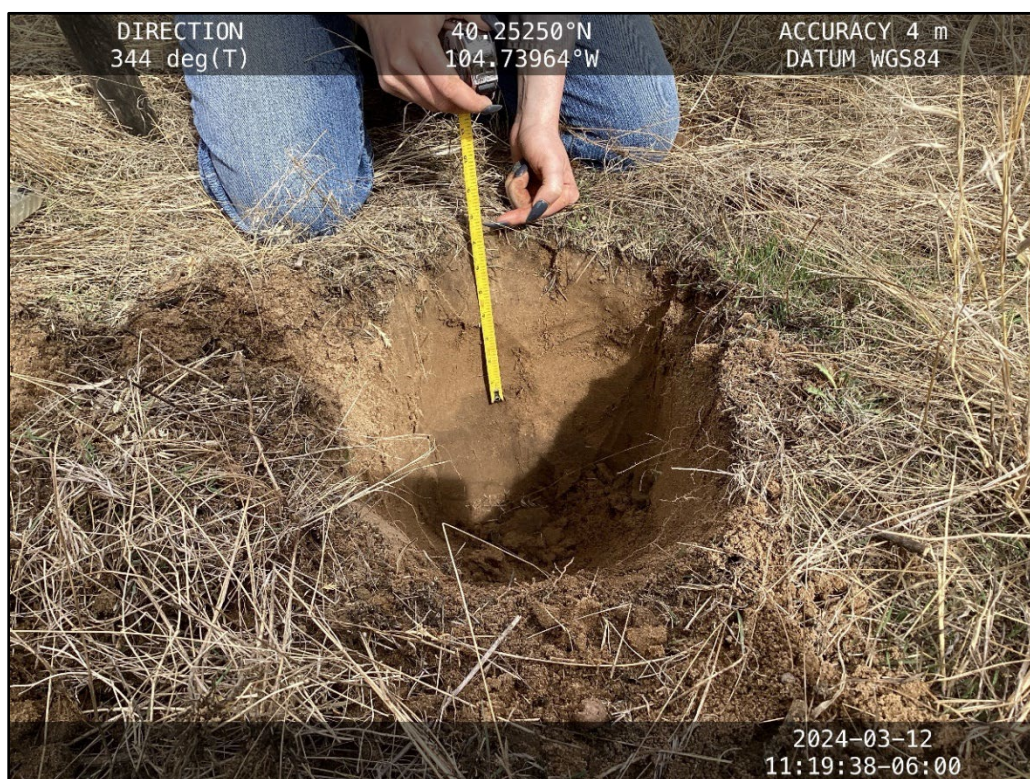
Photograph 4. Topsoil depth pit (CS04) – showing a change in color and composition at 7.5 inches .
