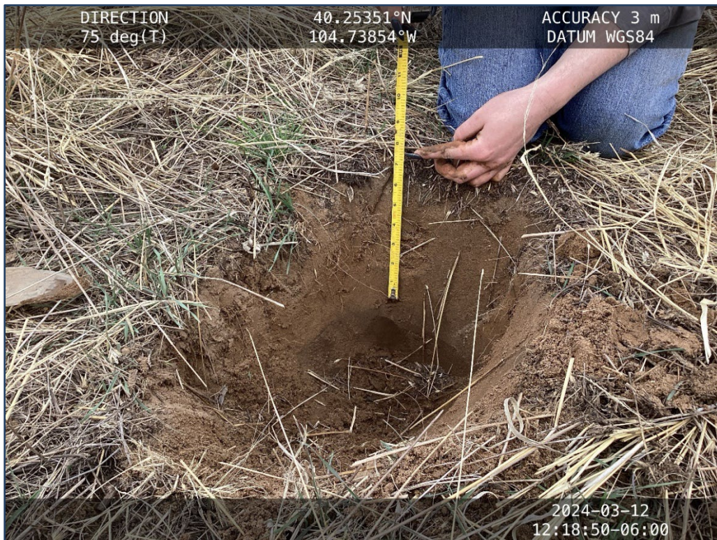
Photograph 2. Topsoil depth pit (CS02) – showing a change in color and composition at 7.5 inches .
