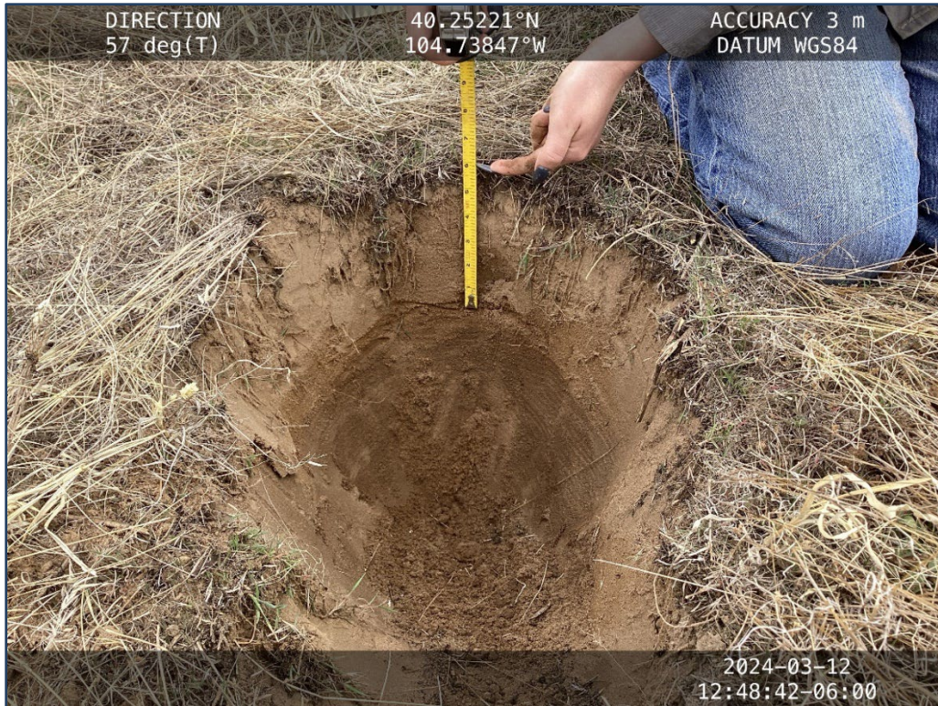
Photograph 5. Topsoil depth pit (CS05) – showing a change in color and composition at 6 inches .
