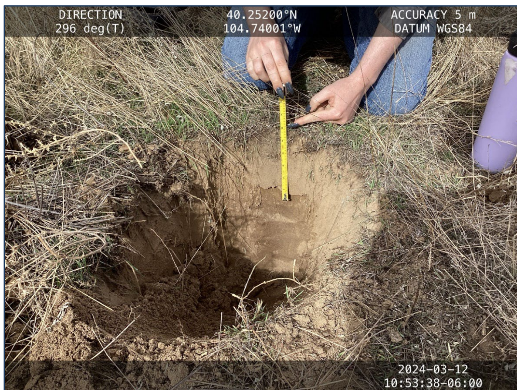
Photograph 7. Topsoil depth pit (CS07) – showing a change in color and composition at 6 inches .
