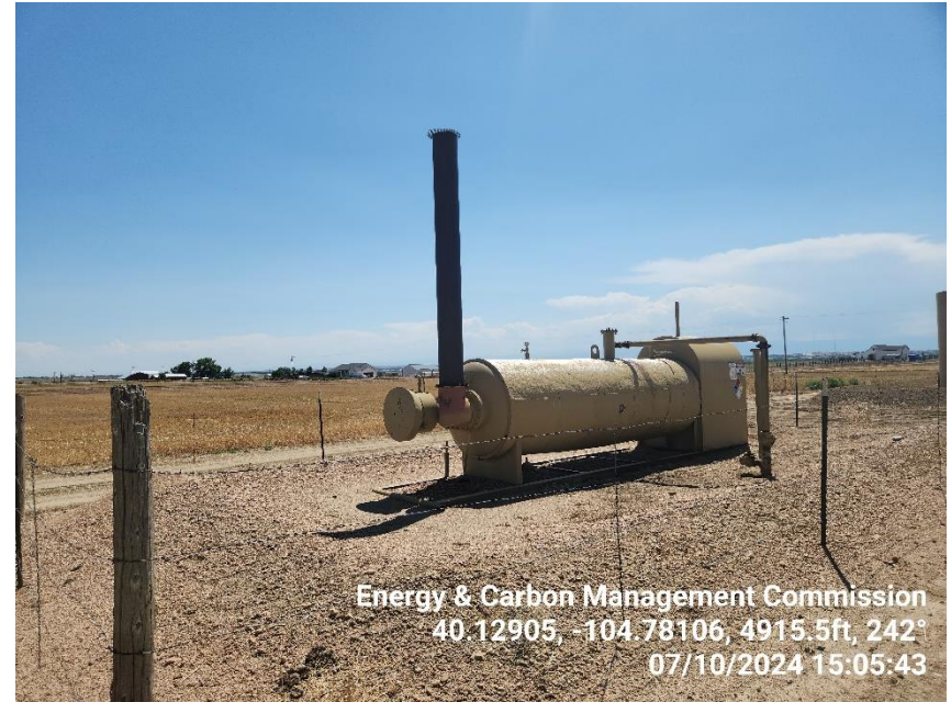
Photo 12 Horizontal heated separator.
