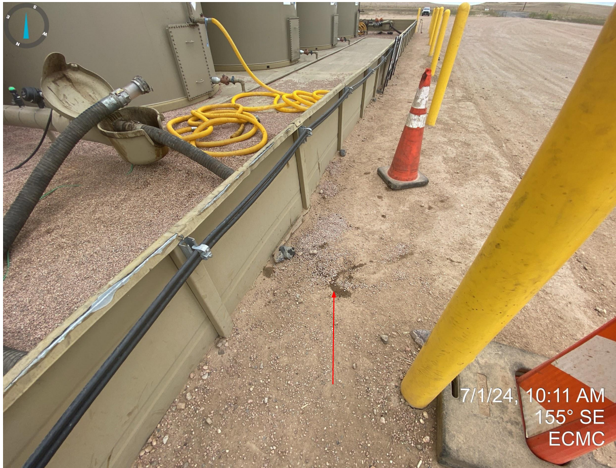
Photo 20. Stained soil observed on west side of tank battery.
