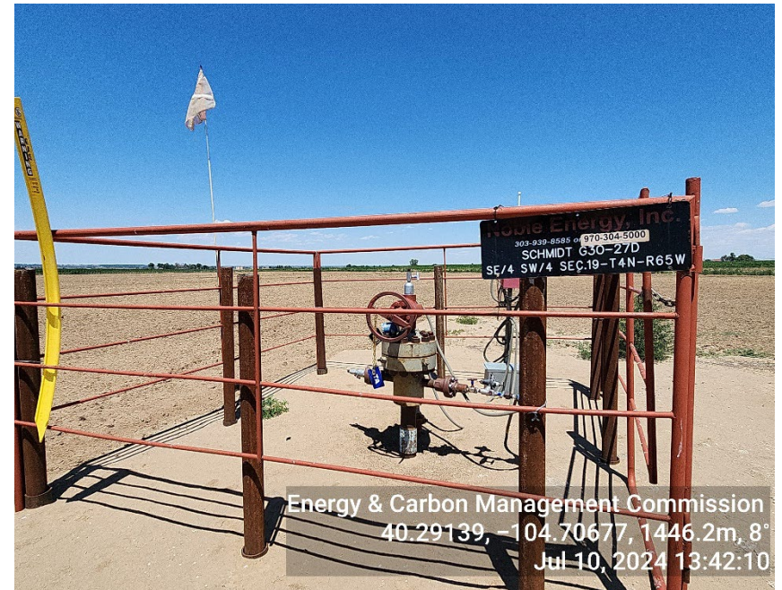
Photo 4: TA wellhead
