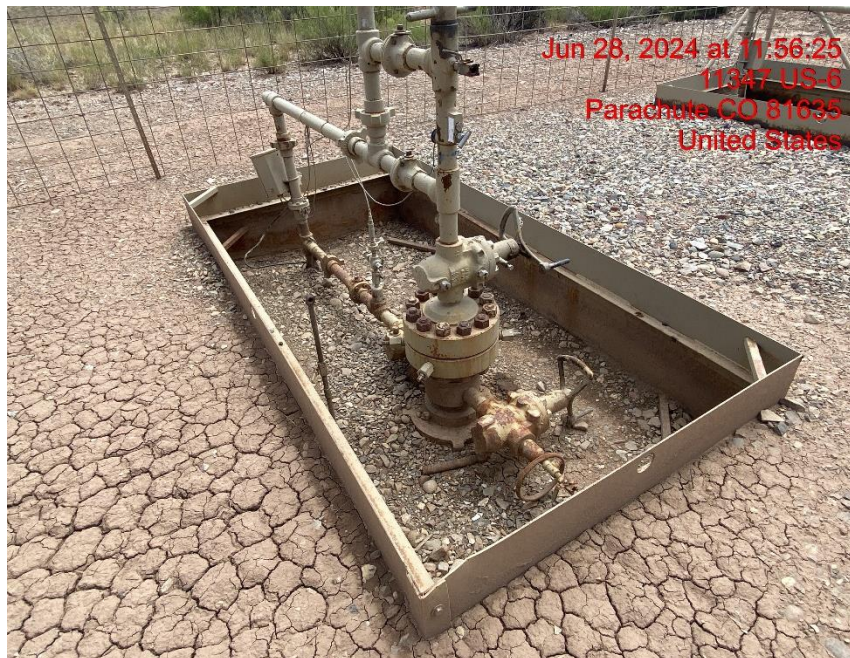
Open Wellhead Cellar – Photo #02120
