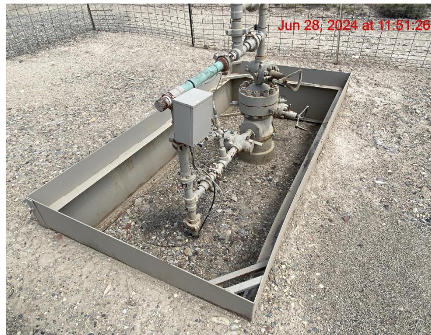
Open Wellhead Cellar – Photo #02115
