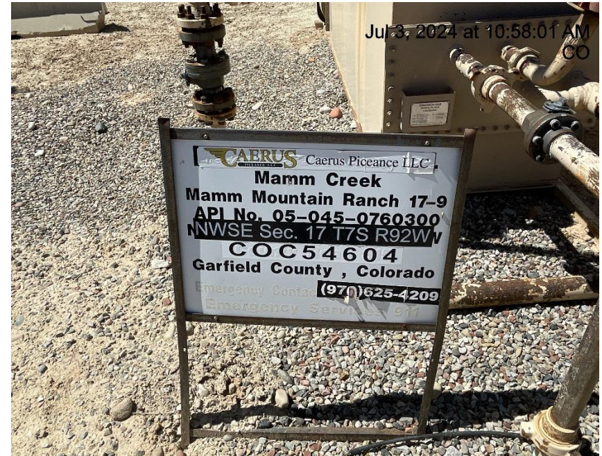
Photo # 2432 Some info on wellhead sign faded & becoming illegible & emergency contact # peeling
