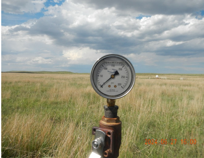
3. Tubing pressure at time of inspection.
