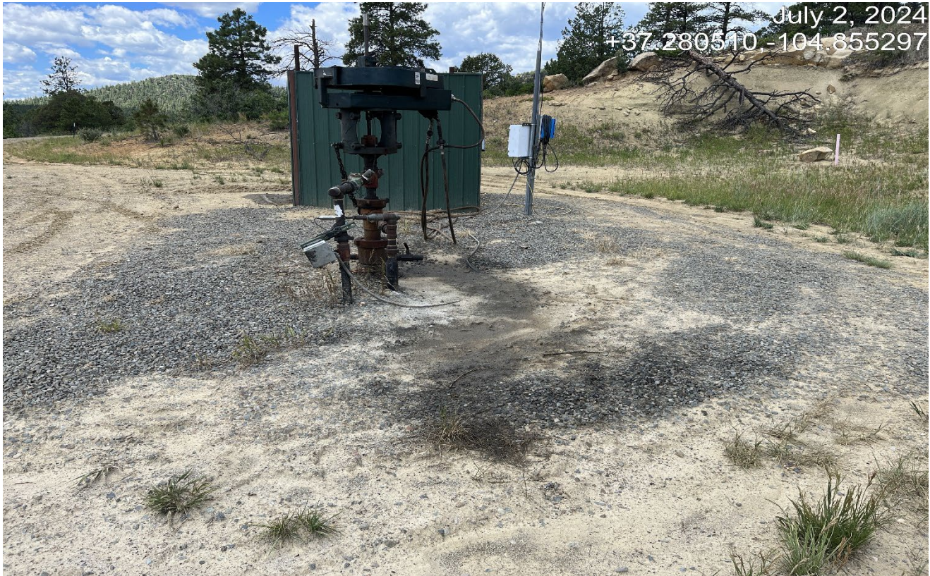
Photo 4. There is stained soils by the wellhead that needs to be cleaned up.
