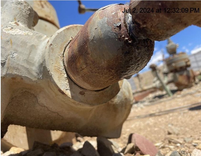
Photo # 2225 Mechanical Condition – possible leak on bullplug connected to RWF 432-26 well casing valve
