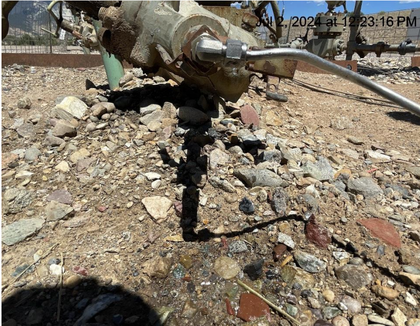
Photo # 2221 Mechanical Condition – possible leak on chemical line connected to RWF 432-26 well casing valve
