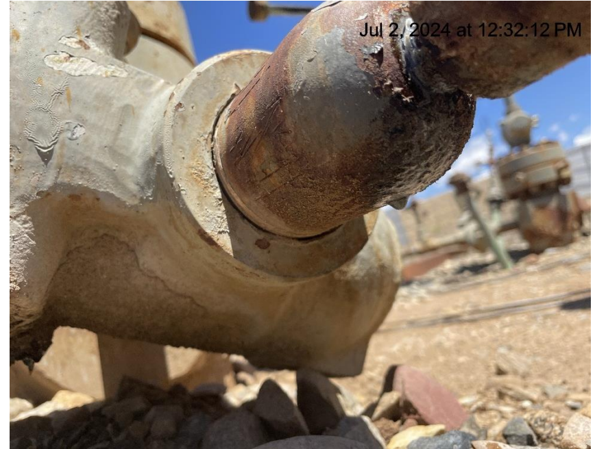
Photo # 2226 Mechanical Condition – possible leak on bullplug connected to RWF 432-26 well casing valve
