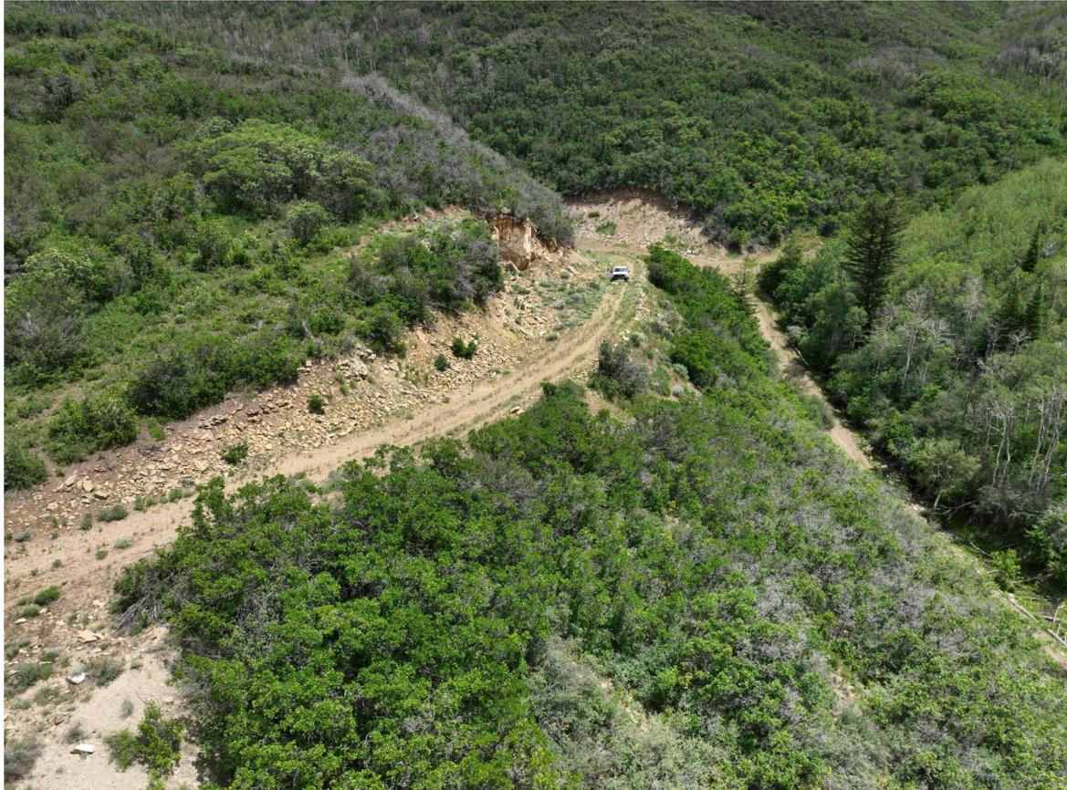
**Photo 5:** Continued from photo 4. Aerial image showing access road has not been recontoured/regraded and reclaimed in accordance with 1004 Rules.
