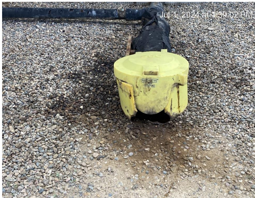
Staining. Pot is now debris. Oil inside and open to wildlife.
