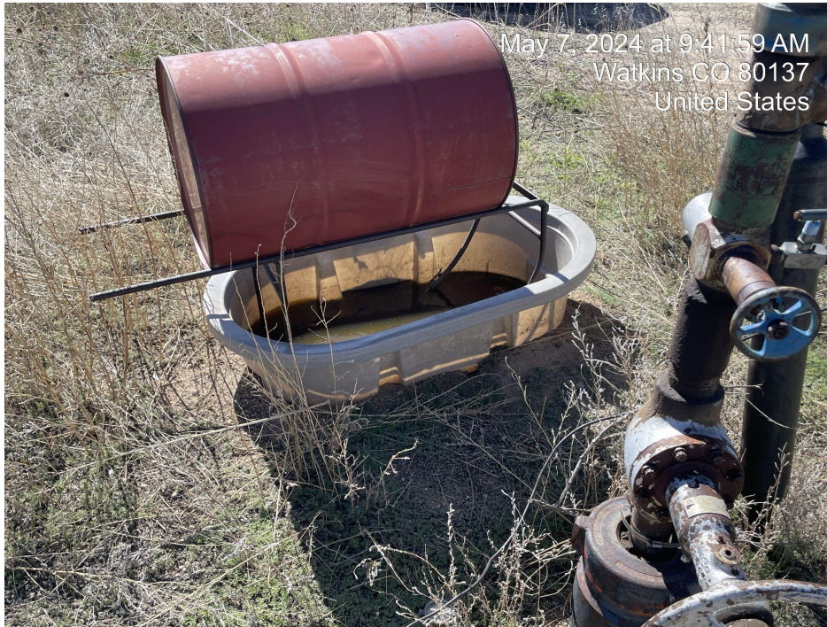
Photo 3. Photo taken facing northeast of barrel on a stand and secondary containment.
