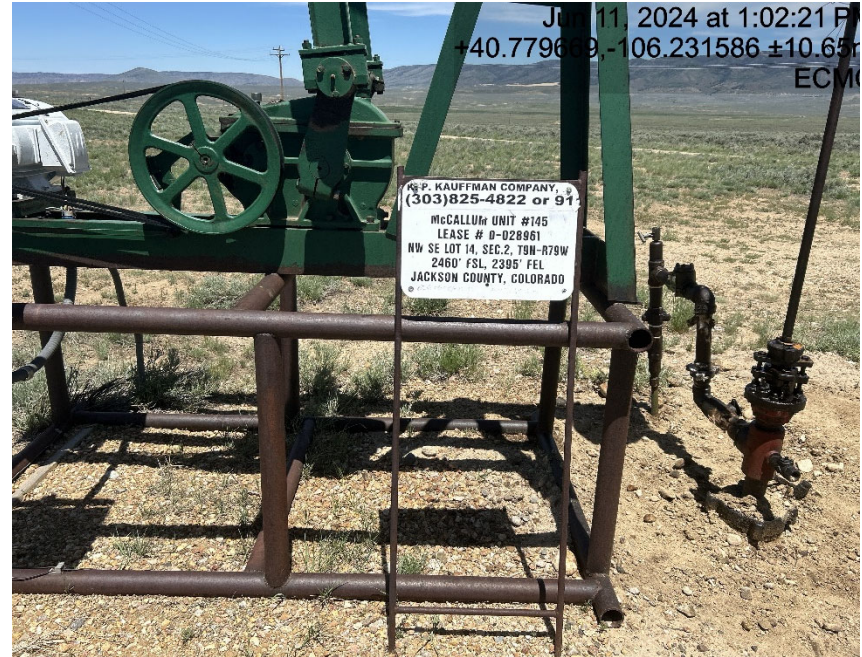
Missing/illegible information on well head signage
