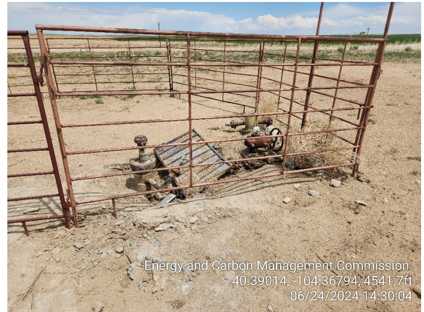
Photo 8 – Antelope F-19 Nightcap – Plugged waiting on Cut and Cap
