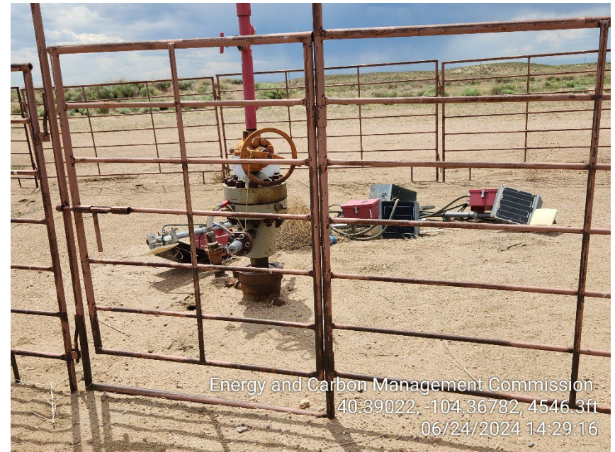
Photo 4 – Wellhead – Unused Automation Equipment
