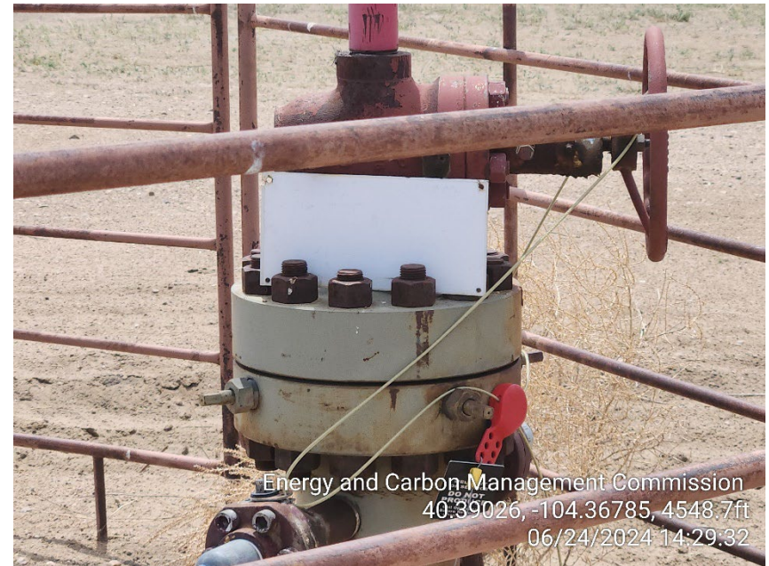
Photo 6 – Wellhead Sign – Faded no longer visible
