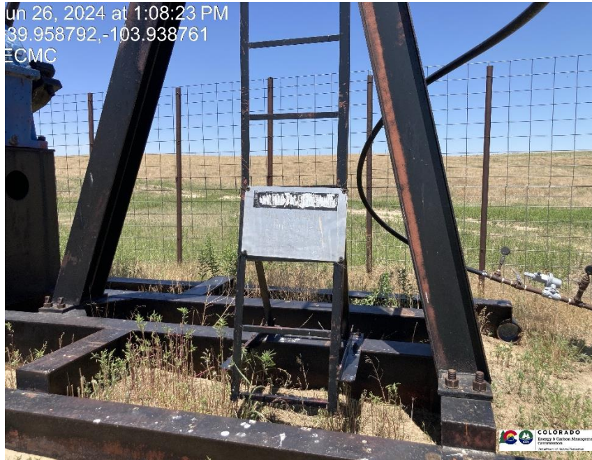
Pic 3 wellhead sign is inadequate
