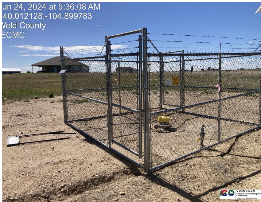
Pic 1 wellhead, well has been PA
