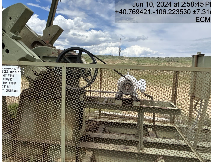
Belt guard is missing
