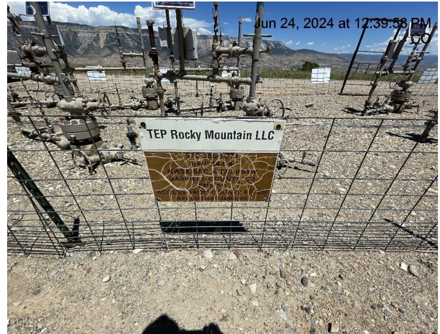
Photo # 1293 Wellhead sign weathered & cracking/starting to become illegible
