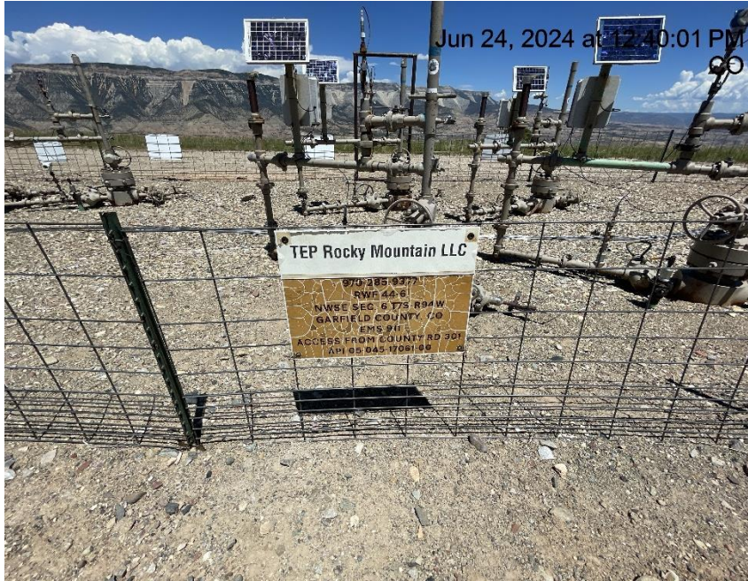
Photo # 1294 Wellhead sign weathered & cracking/starting to become illegible
