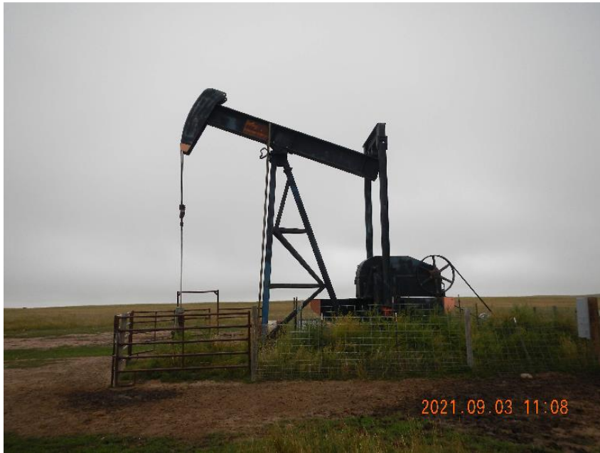
Photo 15: View of Pumping unit, polish rod, and bridle. Note vegetation inside fencing.
