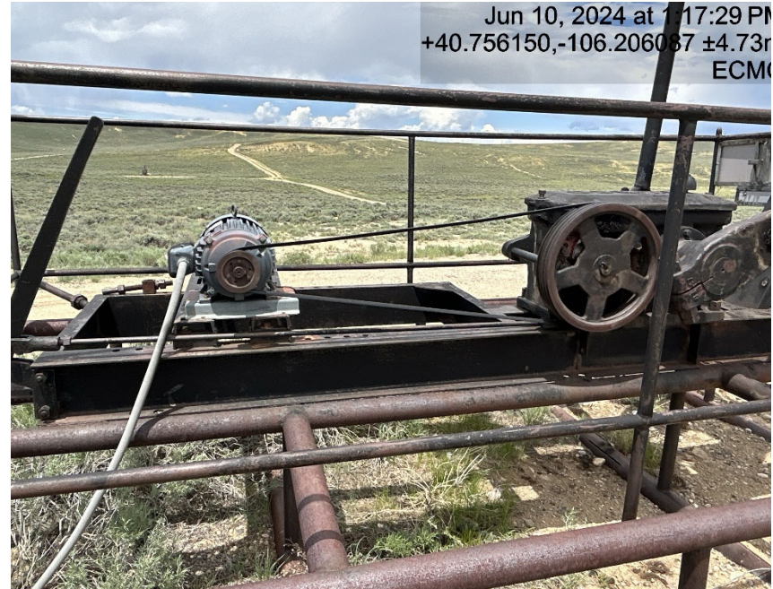
Belt guard missing on pump jack
