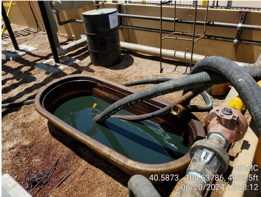
Photo 5 Stock holding condensate/oil/water, No wildlife BMPs, Spills around stock tank
