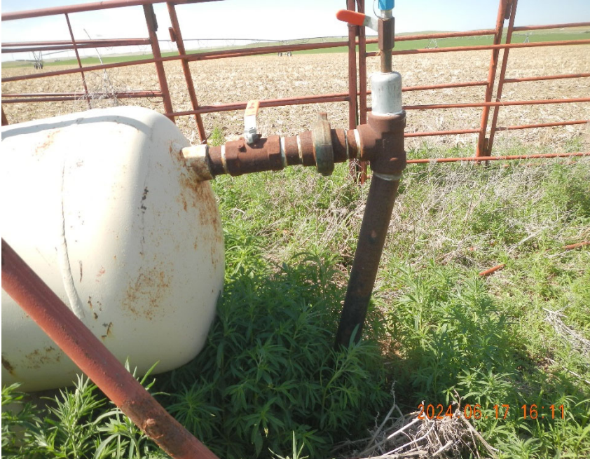
3. Flowline into separator.
