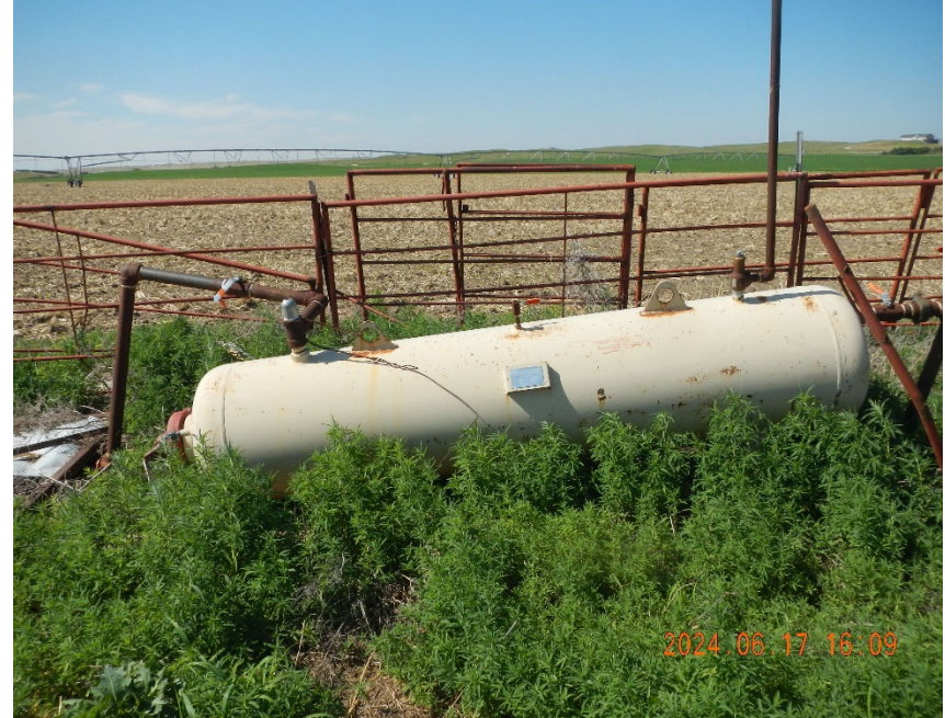
2. Horizontal Separator at well location. Separator is off footings.
