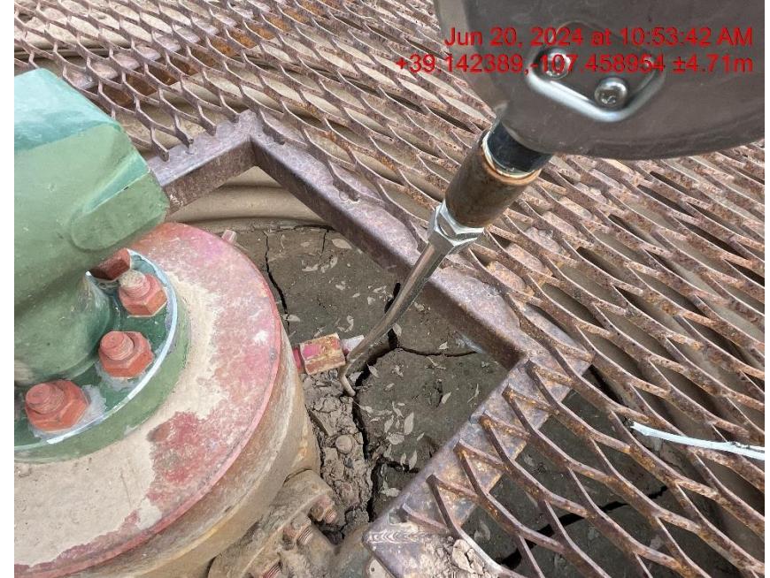
No access to bradenhead valve - Photo #02749
