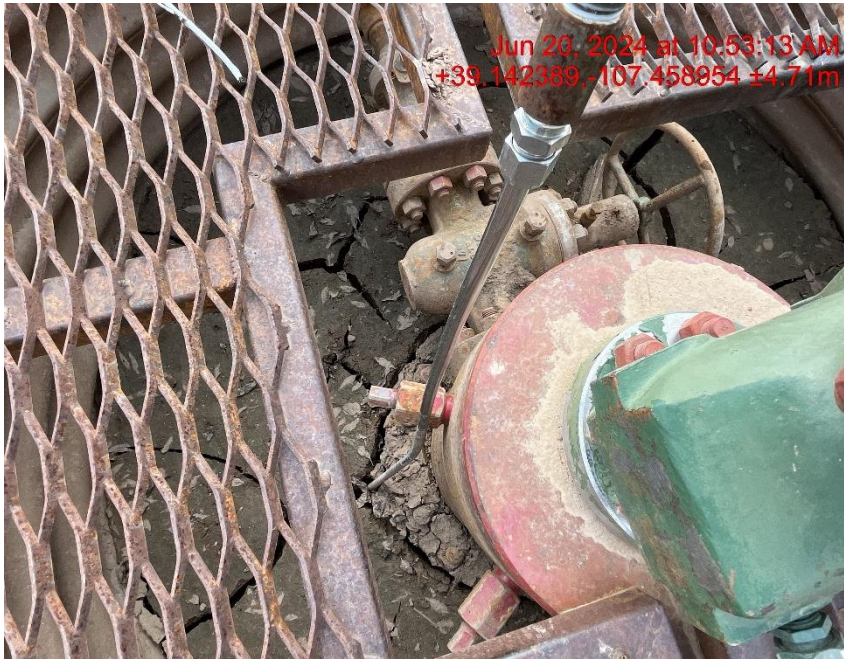
No access to bradenhead valve - Photo #02748
