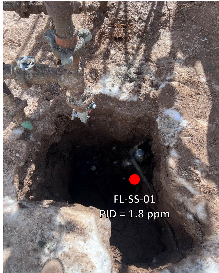
Looking south at flowline Pt B/terminus at separator No petroleum hydrocarbon staining or odor observed
