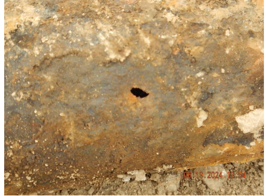
External corrosion pitting identified on the 3" CS flowline pipe segment. It appears external coating deterioration over a long period of time resulted in the failure.
