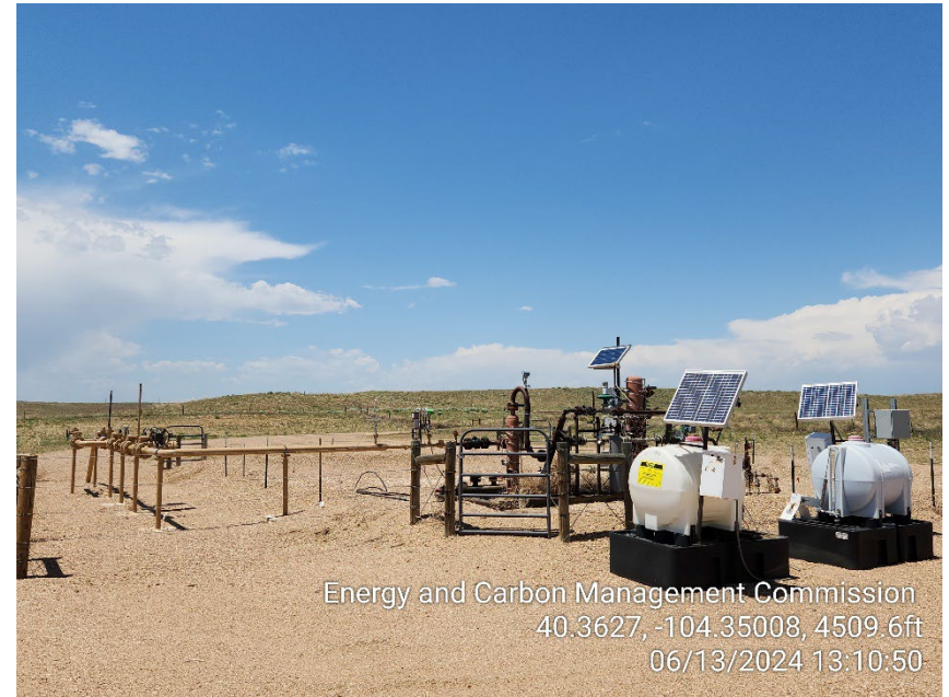
Photo 6 – Gas Lift Injection Meters
