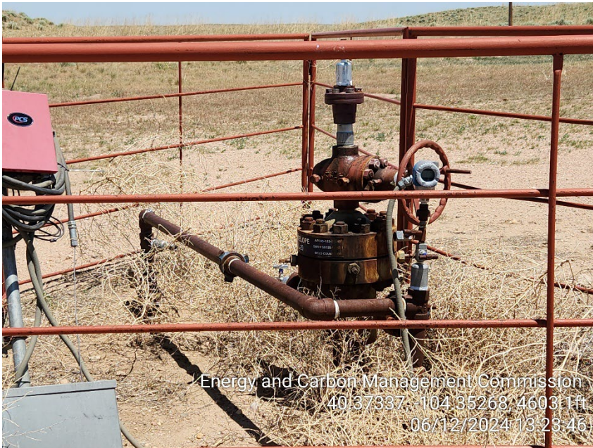
Photo 7 – Wellhead – Tumbleweeds
