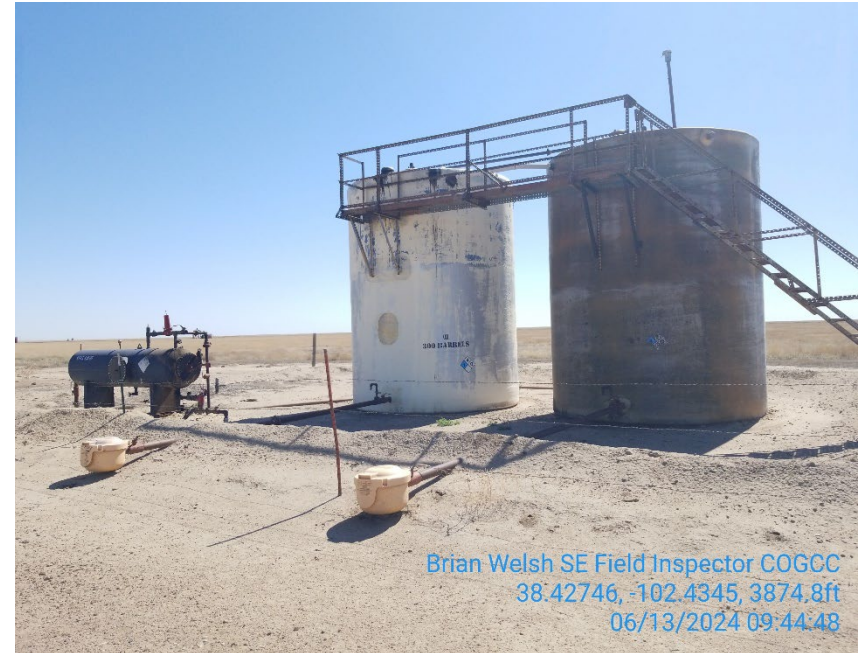
Tank battery and FWKO
