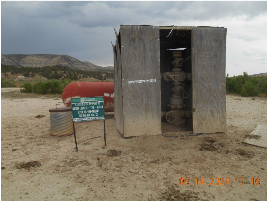
Injection wellhead inside housing
