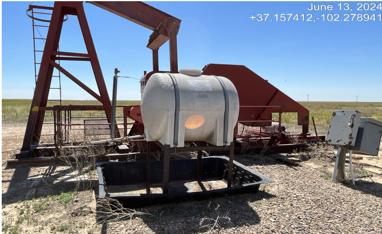
Photo 2. The chemical tank has no lid or labels but appears to be unused and needs to be removed.
