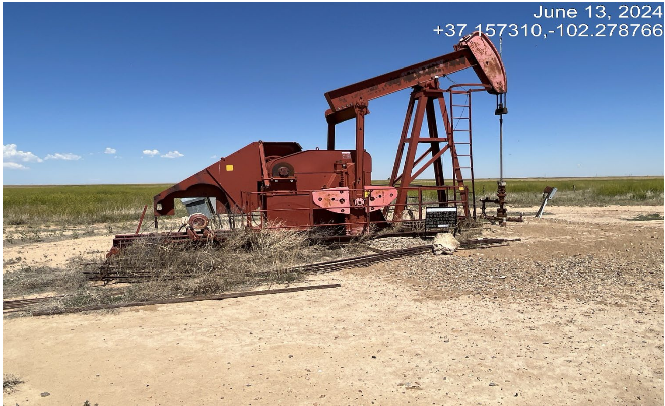
Photo 1. Facing toward the wellsite. There is unused pipe laying next to the pumpjack that needs to be removed. The operator name on the sign is faded and needs to be updated.
