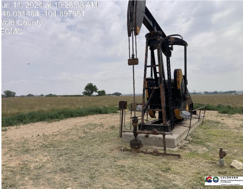
Pic 1 wellhead / pump jack
