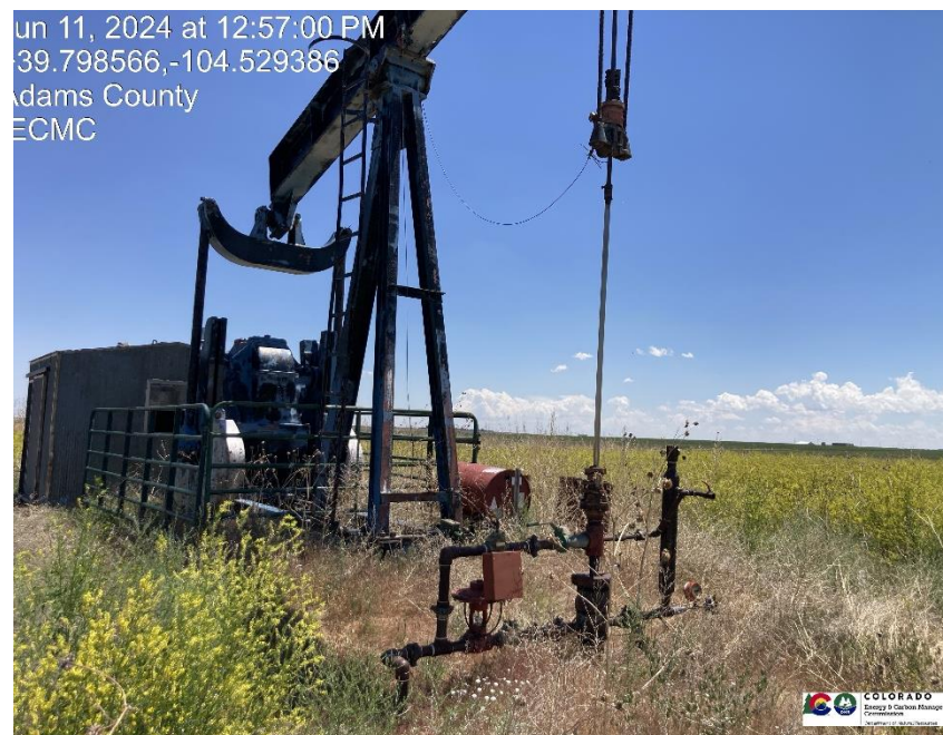
Pic 8 Wellhead / pumpjack
