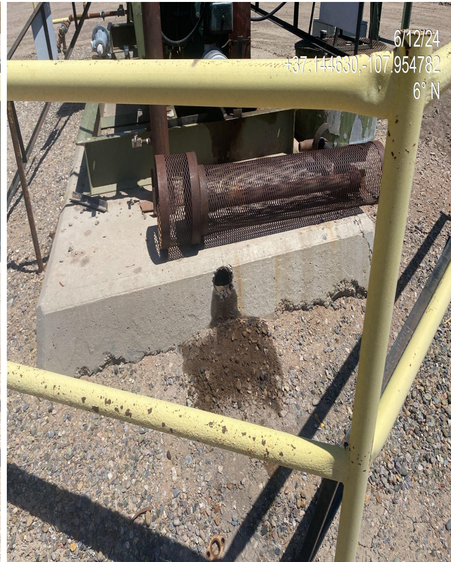
Photo 3. View of impacted surface material observed at the pump jacks.
