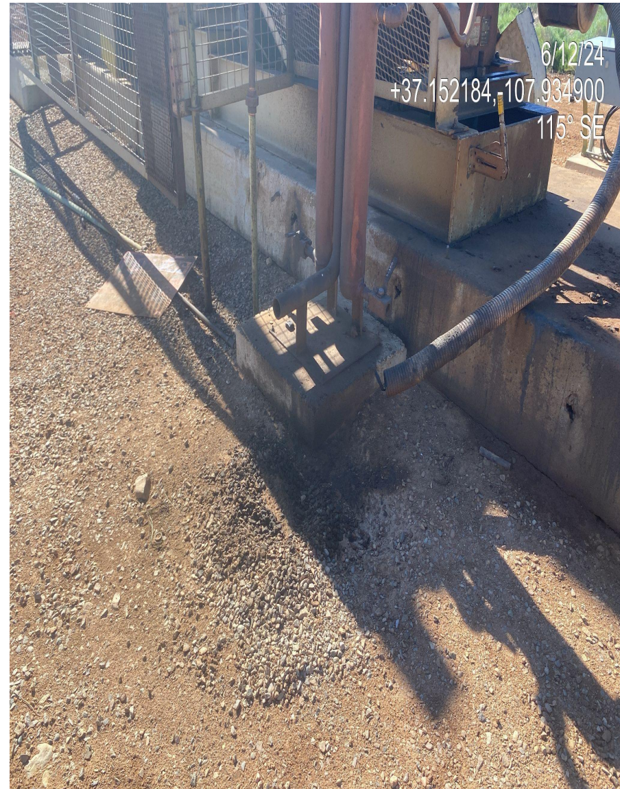
Photo 2. View of stained soils at the pump jack stand and muffer.
