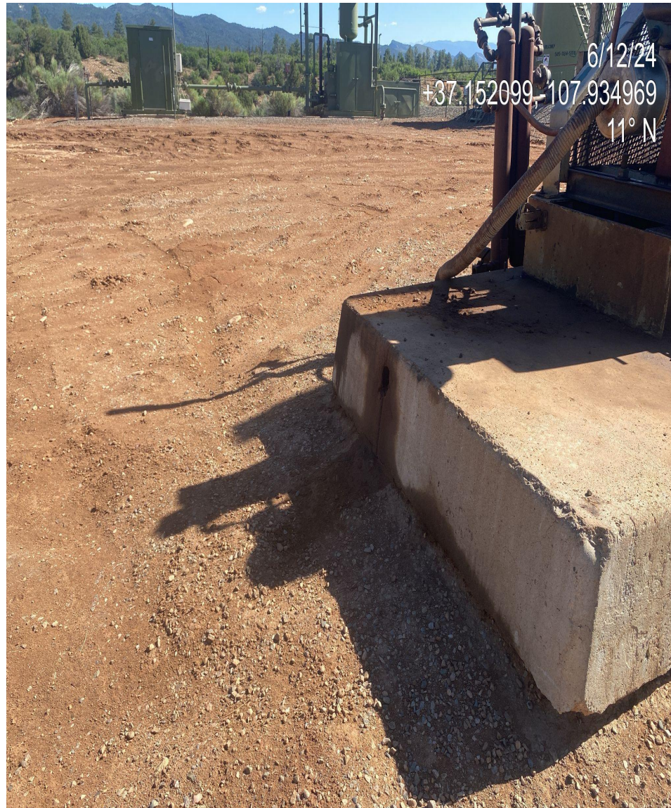
Photo 2. View of stained soils at the pump jack stand and muffer.
