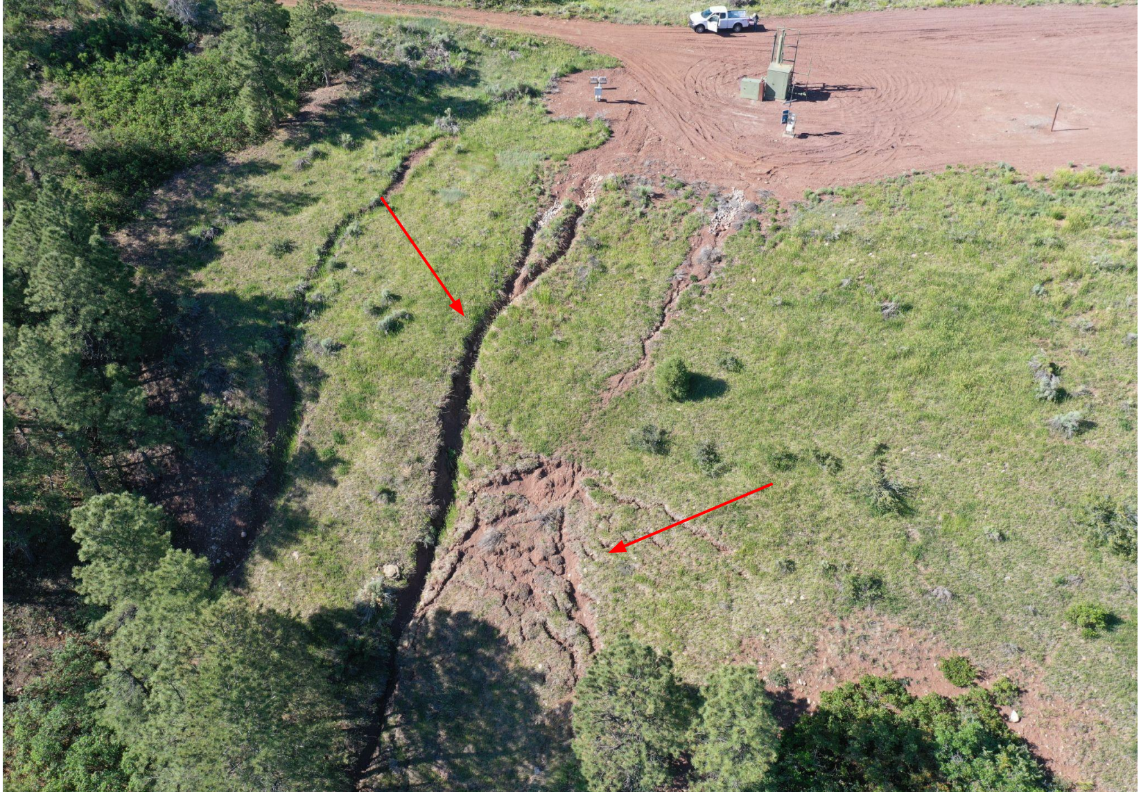
Photo 3. Additional view of gully erosion and sloughing occurring in the northern interim reclamation area. Additional stabilization is needed in this area. Photos taken with a drone from the northern edge facing south.
