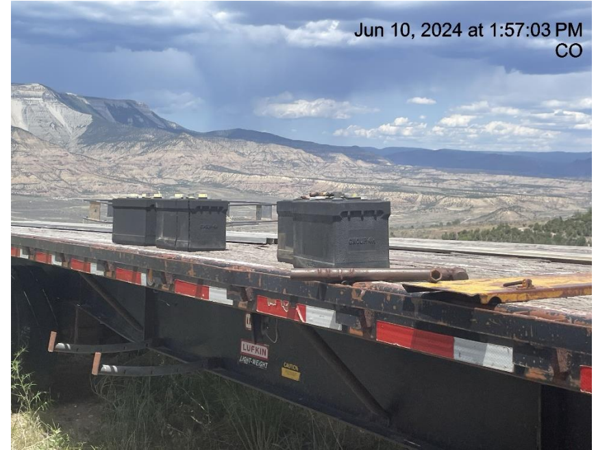
Photo # 309 Improperly stored batteries
