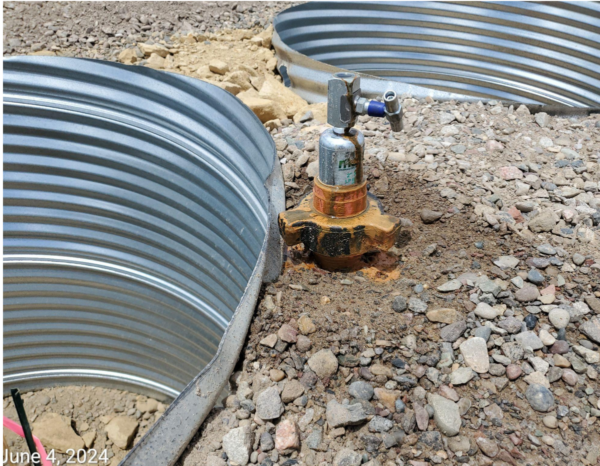
Photo 3: Photo example showing riser equipment leaking fluids; several leaking risers observed on Location.
