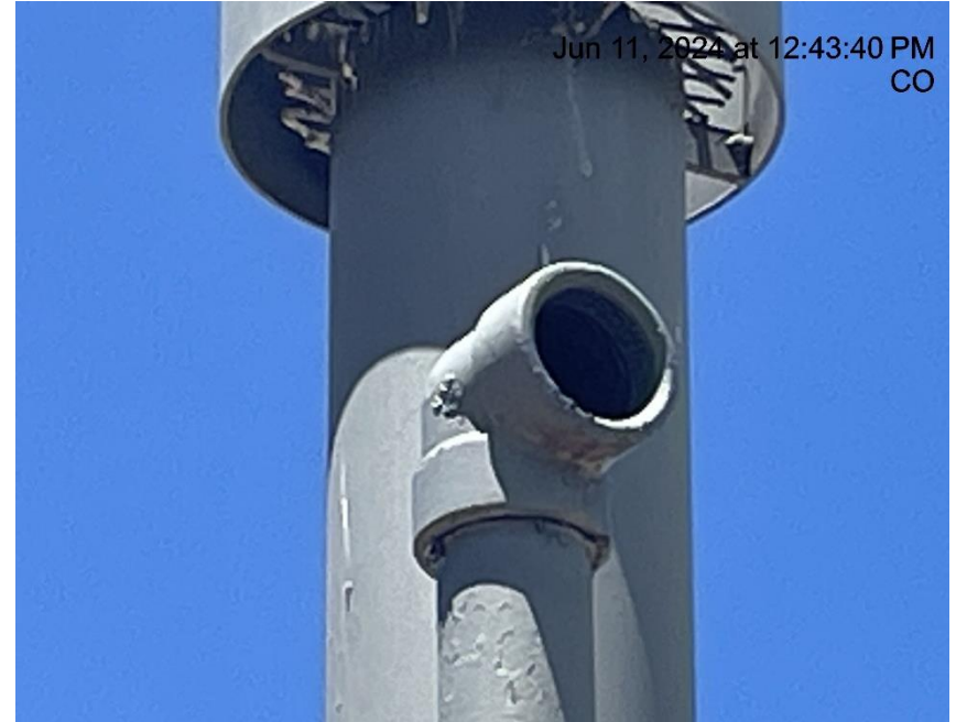
Photo # 507 Open ended piping on separator/wildlife hazard/available for entry by wildlife
