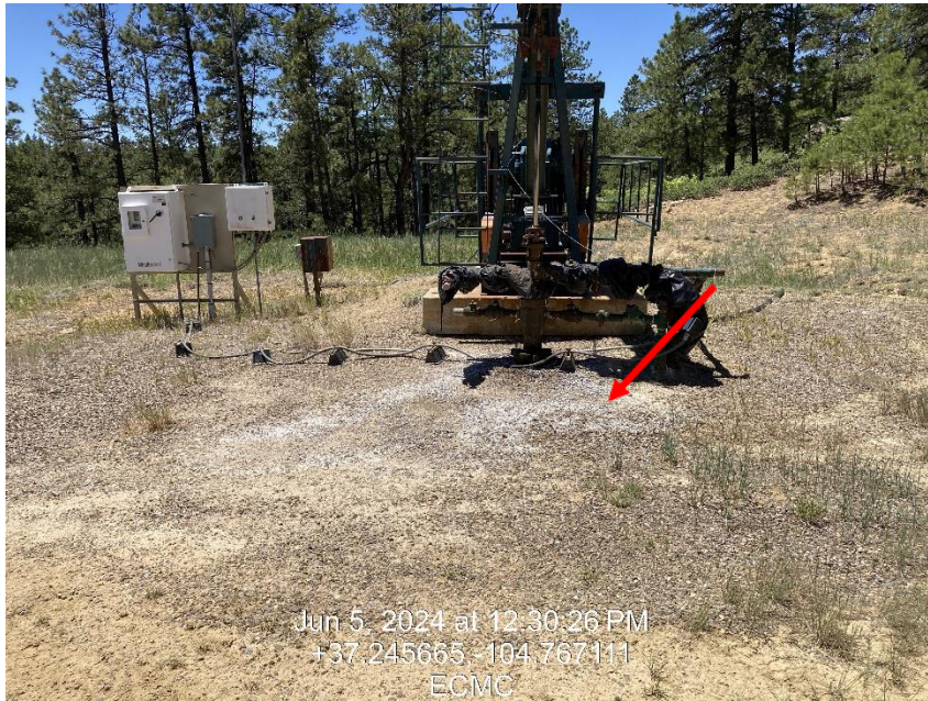
Photo 3 – KV Wellhead, White stained soils
