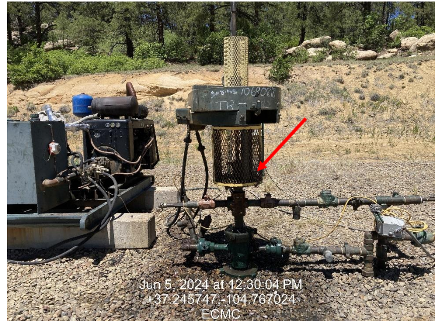
Photo 4 – TR Wellhead, Packing leak, Notified ENR Foreman
