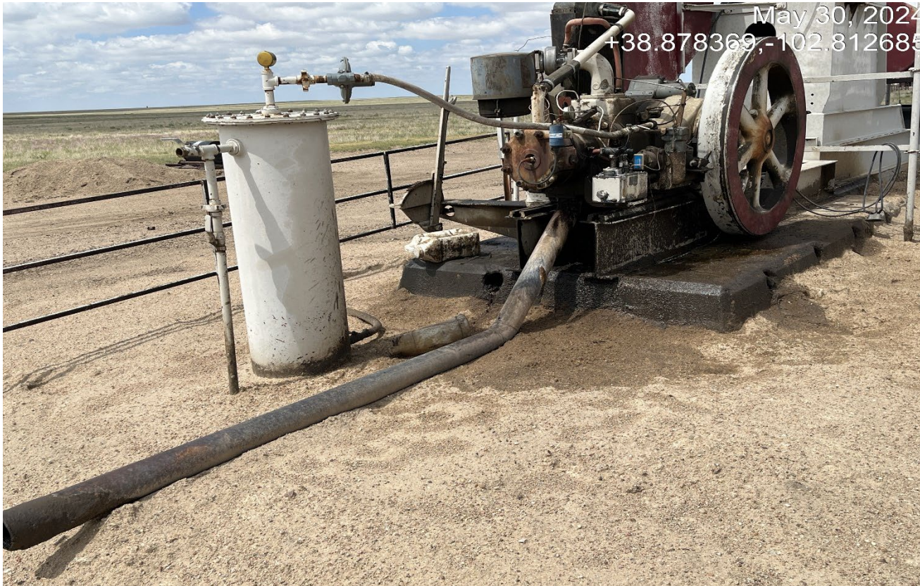
Photo 6. The pumpjack engine is still leaking oil.
