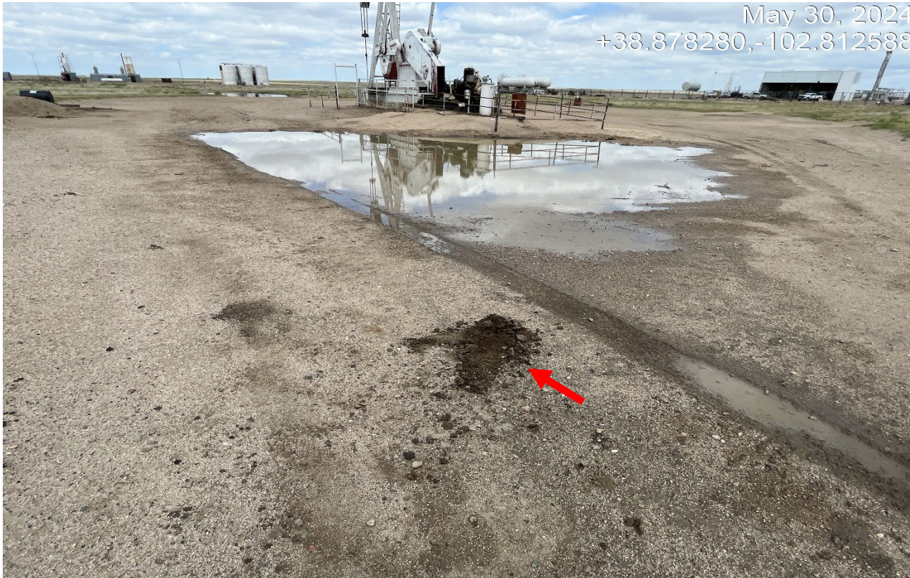
Photo 5. Facing northwest toward the wellsite. The red arrow points to oily soil spilled in this area.
