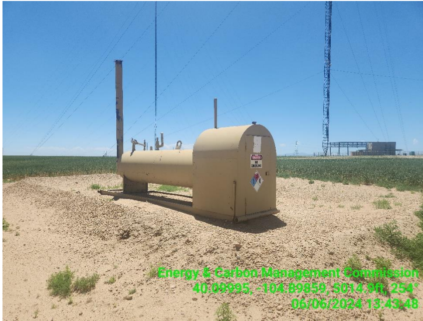
Photo 9 Horizontal Heated Separator.
